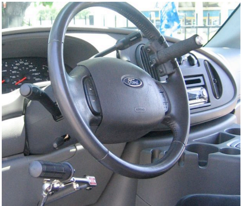
Destinations Mobility vans can be equipped with hand controls for customers who are able to drive themselves.
