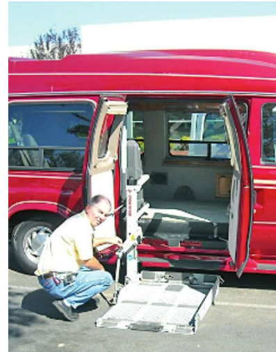
Photo: Richard Rosebush Service Manager Brian Duymich adjusts the wheelchair lift.
